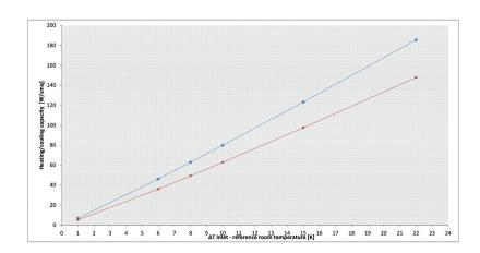
Nota: Efficiency in W/sqm determined by tests in thermostatic chamber according to EN14037 and EN14240.
