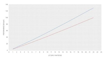
Note: Efficiency in W/sqm determined by tests in thermostatic chamber according to EN14037 and EN14240.
